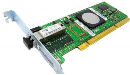
HPE 4GB 1-PORT PCI-X 2.0 FIBER CHANNEL BUS ADAPTER. AB378-60101
