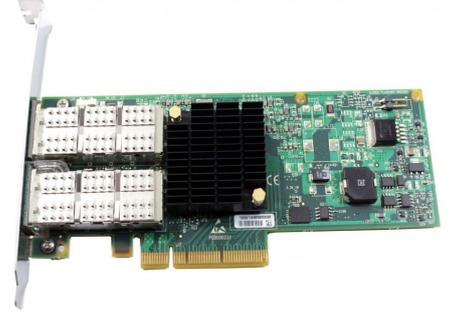
Mellanox MHQH29B-XTR ConnectX-2 VPI Dual QSFP Network Adapter 40Gbps PCI-Express 2.0 x8
