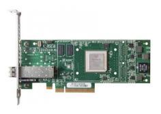
HPE STOREFABRIC SN1000Q 16GB 1-PORT PCIE FIBER CHANNEL HOST BUS ADAPTER. 699764-001 QW971A
